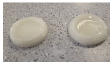
Figure 1. 1:2 Proportion Samples with 7.5 g Castor Oil (Left) With Starch (Right) Without Starch
